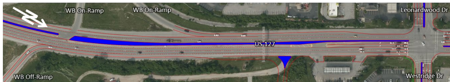
Figure 11: Extra Northbound Thru Lane on US 127
